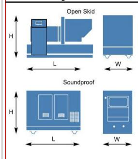
Open Type (Standard Configuration) Overall Size: 6000\*2600\*2800 mm(L\*W\*H) Weight:13500Kgs
